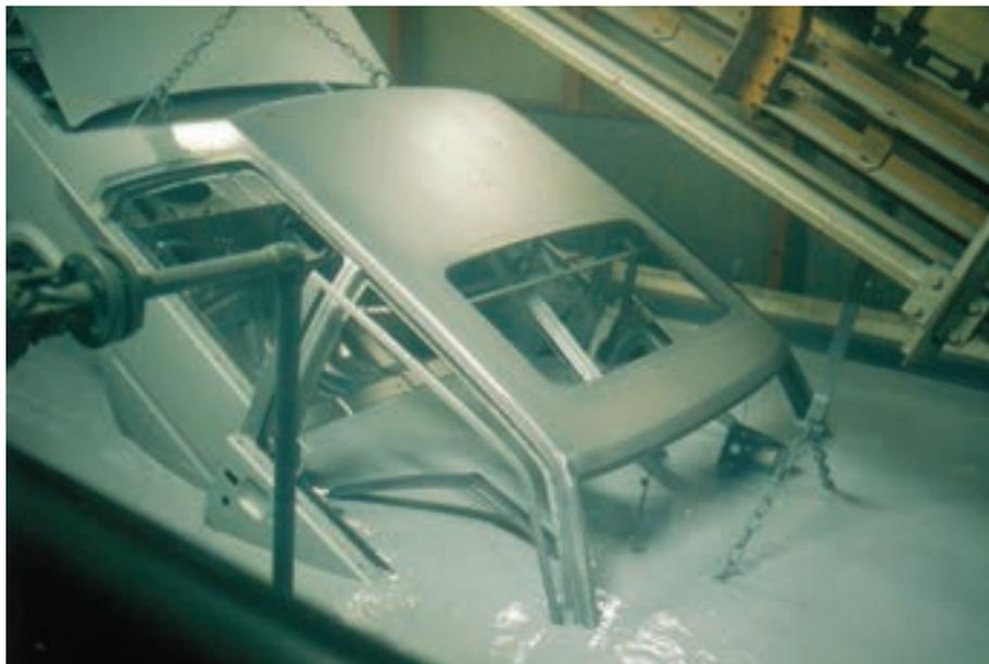
**Pickling a 780 by cataphoresis in the immersion bath. This process was critical for preventing rust.**
